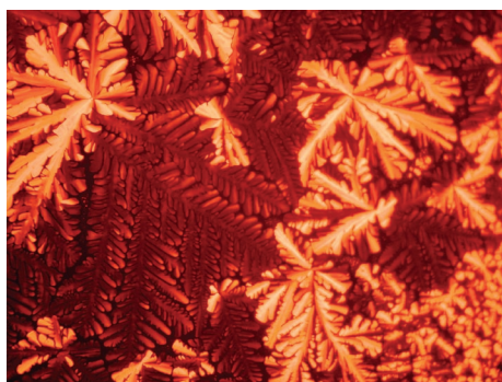
Figure 6. Optical texture of dye 2 between two crossed polarizers obtained by cooling the sample from isotropic phase.
